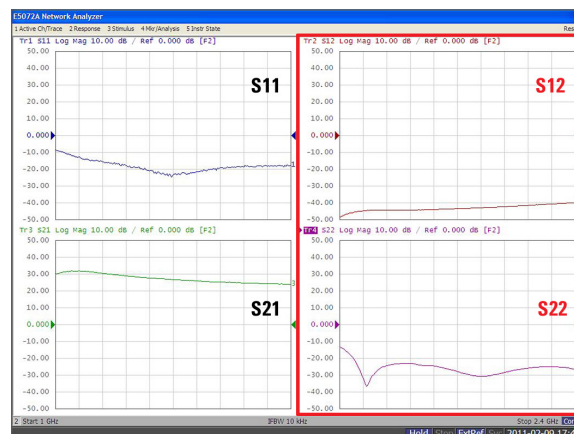
Uncoupled power (Port 1 = -40 dBm, Port 2 = 0 dBm)
