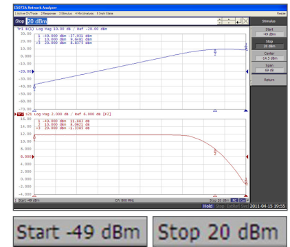
Figure 3. Widest power sweep range in class (ex. settable from -49 dBm to +20 dBm)
